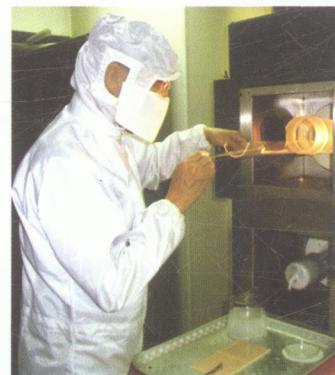
*Inside the high-temperature furnace, high-quality silicon dioxide is grown for the transistors on the silicon wafers, which consist of hundreds of micro-chips apiece.*
