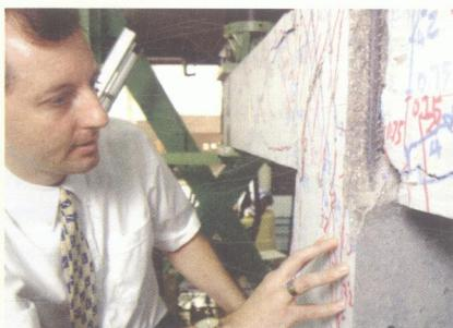
Professor A.M. Chandler inspecting damage to a reinforced concrete beam column joint subject to earthquake action in the laboratory.
