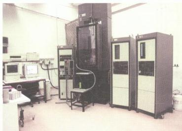
MTS triaxial compression testing machine (capacity 4500kN) for testing rock samples
