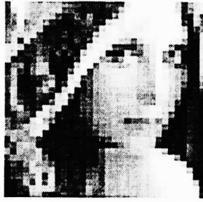
Fig. 7a. Low resolution 32 x 32 image from the (0,0) sensor.
