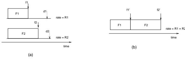
Fig. 5. (a) Rate based scheduling; (b) time-division based scheduling.
