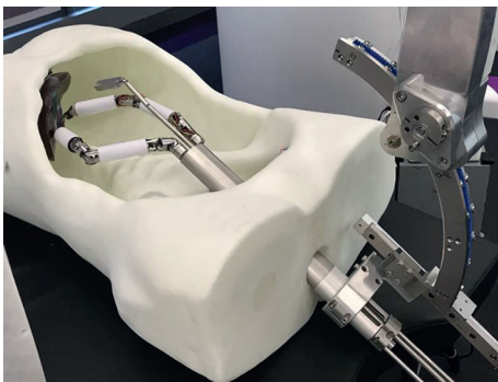
FIGURE 5: Robotic arm and cannula deployment in a female phantom model.
