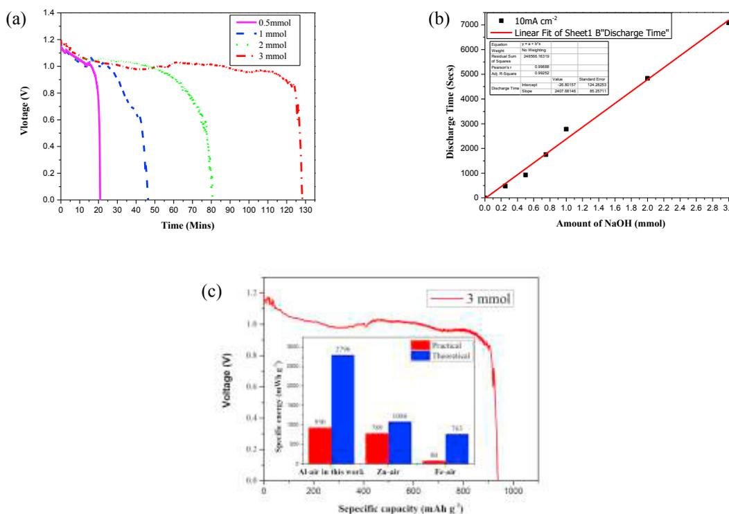
Fig. 5 Parametric study on discharge time for different amounts of NaOH inside the cotton substrate: (a) Galvanostatic discharge at 10 mA cm<sup>-2</sup>; (b) Linear fitting for the discharge time; (c) Galvanostatic discharge (vs capacity) and comparative specific energies.
