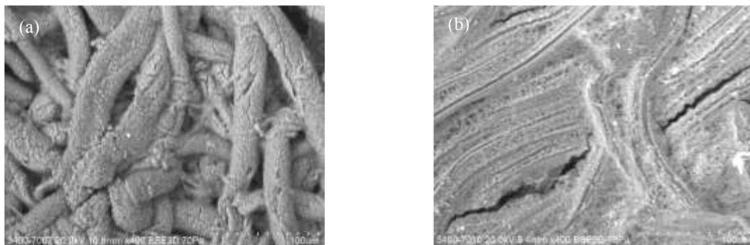
Fig. 4 SEM image of substrate with dry NaOH particles: (a) Cellulose paper substrate; (b) Cotton substrate.
