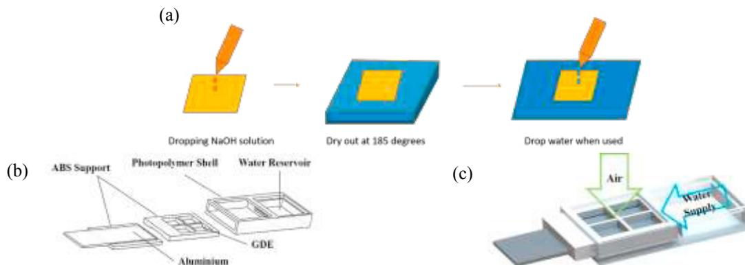
Fig. 1 Schematic diagram of (a) fabrication process of the cotton-based alkaline electrolyte; (b) exploded view of a single battery; (c) assembled battery.
