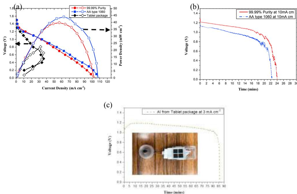
Fig. 2 Performance comparison between different kinds of aluminum: (a) Battery polarization curve; (b) Galvanostatic discharge test using commercial aluminum; (c) Galvanostatic discharge using waste aluminum.
