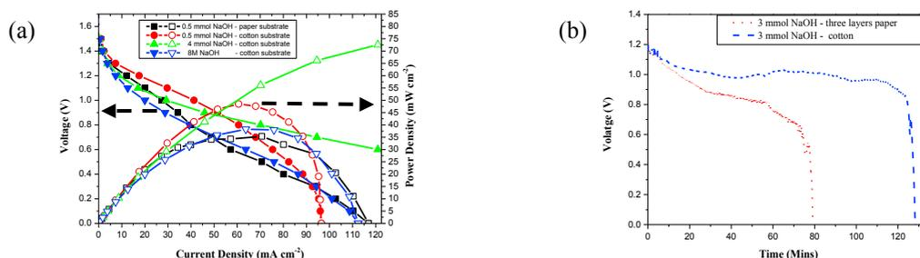
Fig. 3 Performance comparison between different kinds of electrolyte substrate: (a) Battery polarization curve; (b) Galvanostatic discharge at 10 mA cm<sup>-2</sup>.
