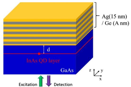
**Fig. 1.** Schematic of the HMM-coupled QD structure under consideration. The green arrow indicates excitation direction, and the purple arrow shows the measurement direction. A thin Ge layer of 2 nm is deposited before HMM deposition.
