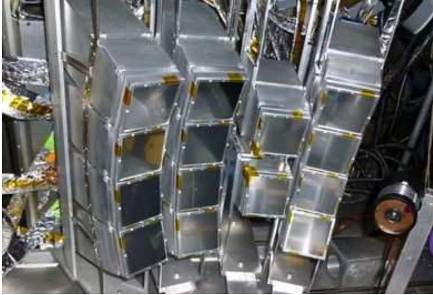
Figure 10: The High Resolution Array (HiRA). In this picture, HiRA is arranged at forward angles for a transfer reaction measurement.
