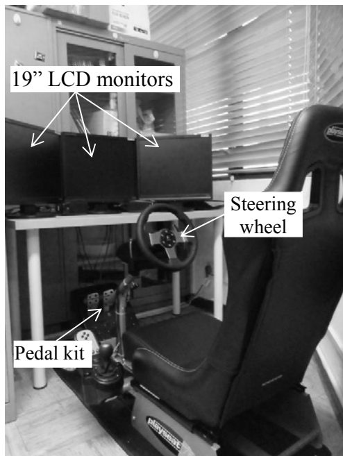
Figure 1 Hardware set up of the driving simulator
