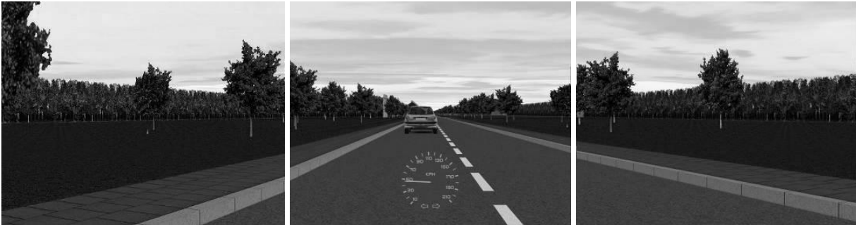
Figure 3b Following braking module at 80 km/h in the simulated driving test
