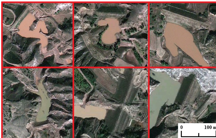
Figure 4. Examples of the sediment-trapping dams identified from the remote sensing images in the Huangfuchuan River basin.
