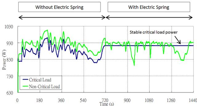
Fig.4 Power consumption of critical and non-critical loads.
