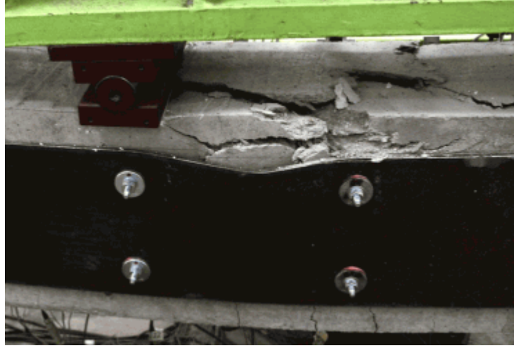
Figure 16. Plate buckling of Specimen P250B300
