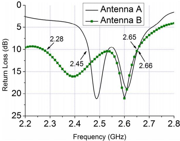
Figure 2. Return loss plots of Antennas A and B.
