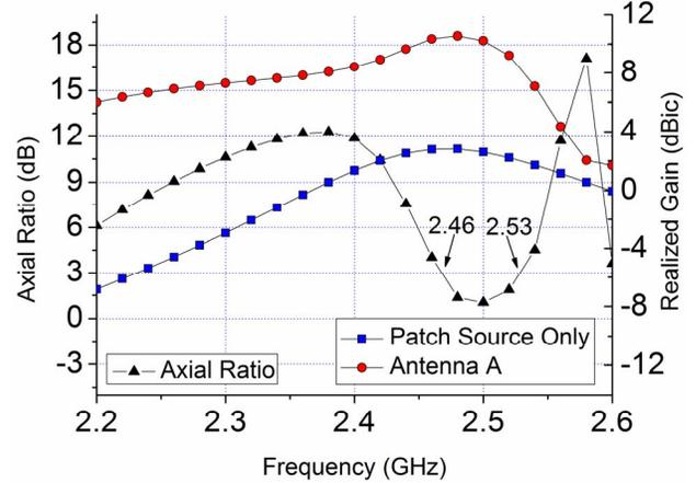
Figure 3. Axial-ratio and gain versus frequency for Antenna A.
