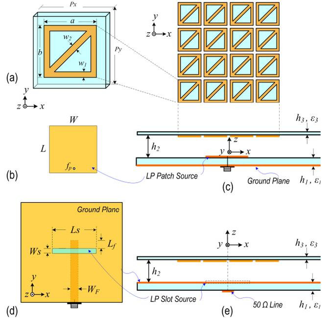
Figure 1. Geometries of the CP metasurfaced antennas: (a) metasurface and its unit-cell; (b)&(c) Antenna A: metasurface excited by probe-fed LP patch; (d)&(e) Antenna B: metasurface excited by line-fed LP slot source.
