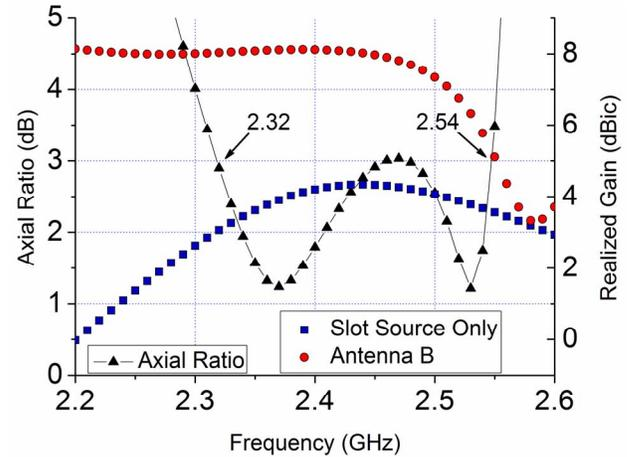
Figure 4. Axial-ratio and gain versus frequency for Antenna B.
