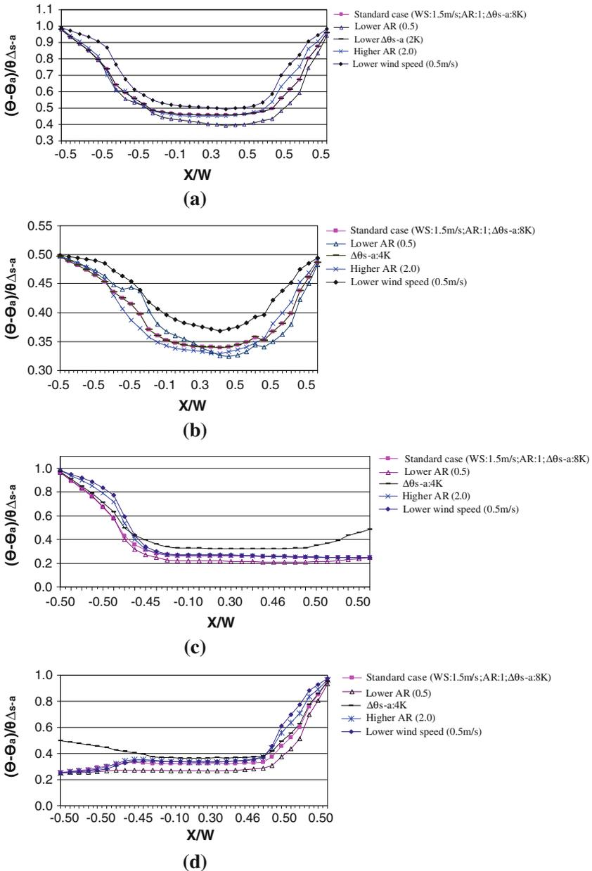
**Fig. 6** Average (area-weighted) normalized air-temperatures along spatial axis of the target (middle) street canyon. Note that different simulation cases are identified with the values different than those for the standard case. **a** Uniform-surface heating. **b** Ground heating. **c** Leeward wall heating. **d** Windward wall heating
