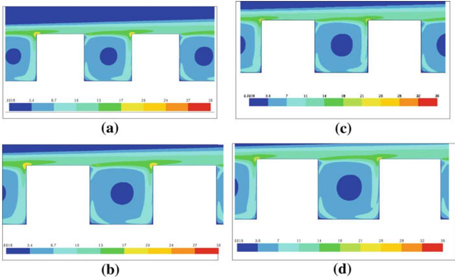
**Fig. 5** Contours of turbulence intensity for the standard case of different heating situations. **a** Uniform-surface heating. **b** Ground heating. **c** Windward-wall heating. **d** Lee-ward wall heating
