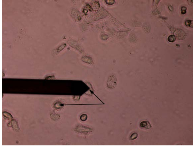
Fig.2c: UM1 cells indented by AFM tip, top view under optical microscope
